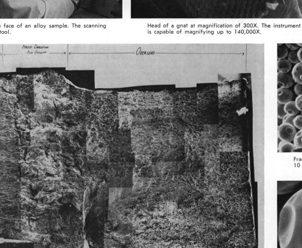
Montage of a fracture face made from 200 separate photos reveals the failure mode of an alloy. The microscope is used
